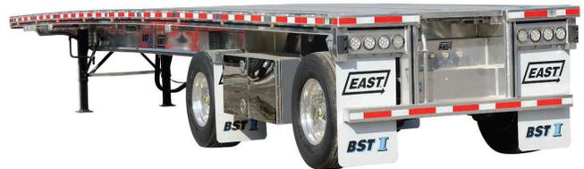
**MMX™** – Offering one of the highest concentrated load ratings in an aluminum flatbed, the MMX is rated to handle loads up to 80,000 lbs. concentrated in 4 feet, up to 89,000 lbs. concentrated in 10 feet and up to 145,000 lbs. distributed with a multi-axle configuration on a 48-foot wide spread trailer. Ideal for multi-axle applications, it is available in lengths up to 53 feet and boasts a 13-inch deep neck with a heavy-duty main beam.
