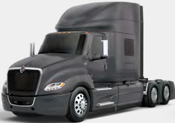
73" Hi-Rise Sleeper 125" BBC Long Haul Flatbed, Owner-Operator and Specialized Applications
